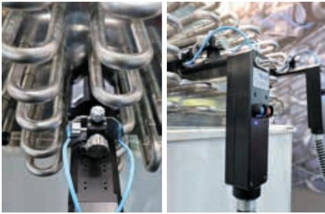
Extremely narrow design - ideal for welding pre-mounted arcs in narrow tube bundles
