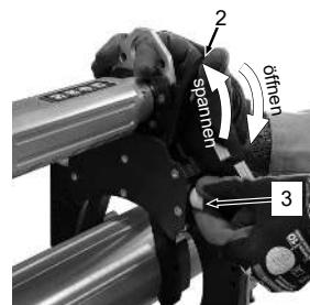
*Fig.: Tighten clamping lever*
