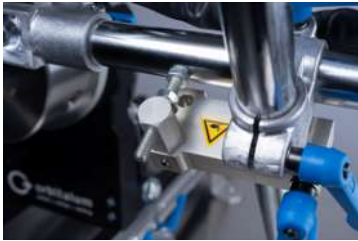
Illustration: Position stop for torch arm
