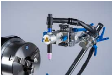
Illustration: Torch holder with joints on cross slide for fine adjustment.
