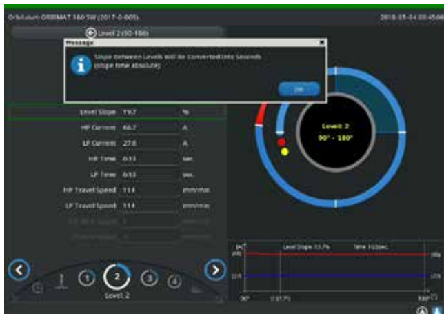
Abb. 12: Converting the slope time from percent to seconds
