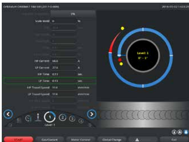
Abb. 13: Input field of a sector with representation of the seam scale
