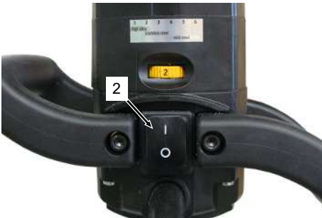
ON/OFF toggle switch on the motor
