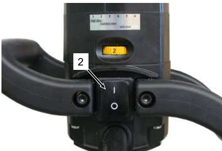
ON/OFF toggle switch on the motor
