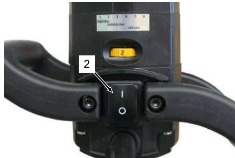
ON/OFF toggle switch on the motor
